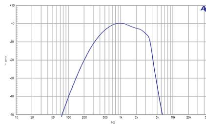
Figure 9. FIL-CIT. CCITT P53 Noise Weighting Filter.
