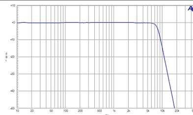
Figure 19. 8 kHz 7-pole Low Pass Filter.
