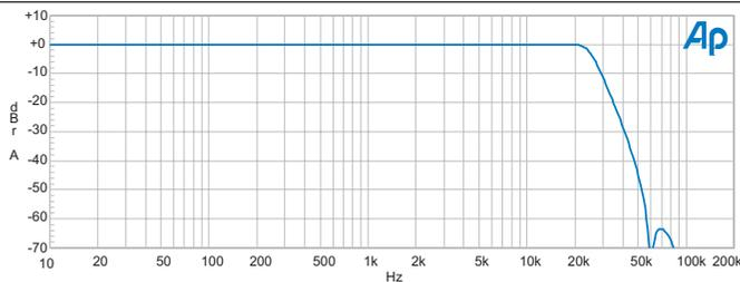
Figure 25. Typical response of 20 kHz “pre-analyzer” filter.
