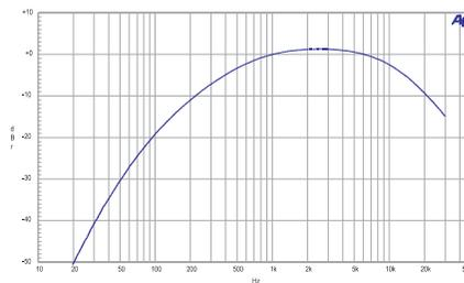
Figure 7. FIL-AWT. ANSI-IEC “A” Weighting Filter.
