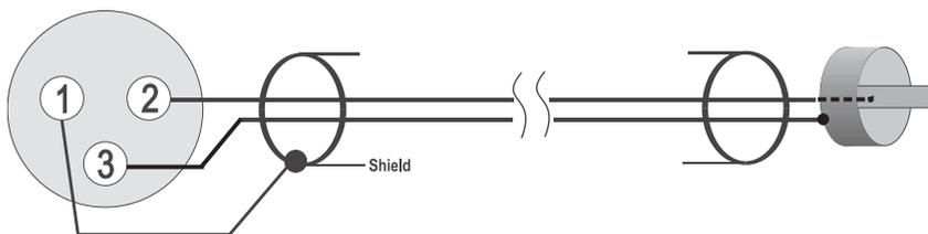
Figure 36. XLR to BNC wiring
