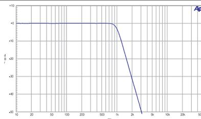
Figure 18. 1 kHz 5-pole Low Pass Filter.
