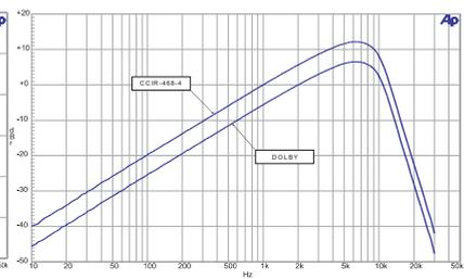
Figure 8. FIL-CCR. IEC468 (CCIR)/DIN 45404 Noise Weighting Filter.
