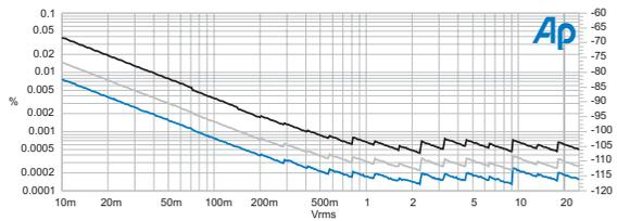
Figure 2. Typical system THD+N versus amplitude at 1 kHz. Lower trace is with 22 kHz bandwidth limiting. Middle trace is with 80 kHz.
