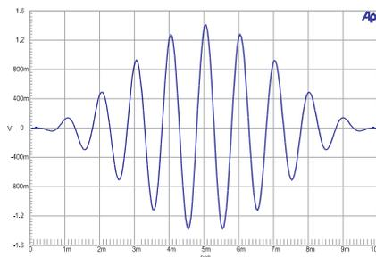
Figure 30. Shaped Sine Burst signal.
