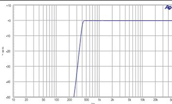
Figure 20. FHP-400. 400 Hz 9-pole High Pass Filter.
