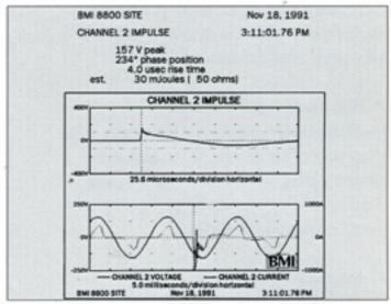
Impulse Graph. When an impulse is detected, the 8800 generates two graphs. The lower graph shows the voltage and the current waveforms before and after the impulse. The upper graph shows the actual impulse, sampled at 4 MHz and automatically zoomed to its best resolution.
