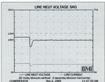
Simultaneous Voltage and Current Graphs. The top graph shows that the offending load is downstream of the monitoring point since an increase in current occurs simultaneously with a decrease in voltage. The graph below shows little or no change in current, indicating the disturbance originates upstream of the monitoring point.
