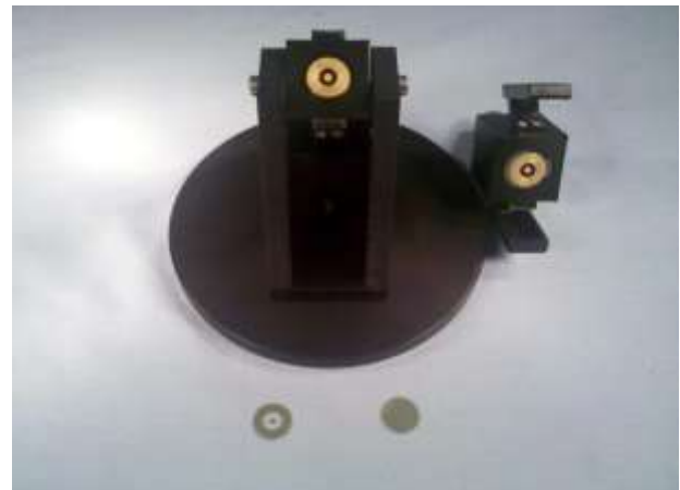
Decoupled Specimen Holder with Gold Reference (left) and Load (right) Inserts in foreground
