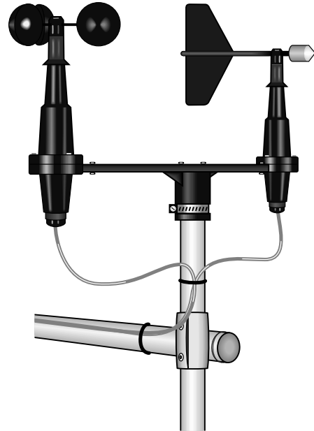
A crossarm and 10" x 3/4" -diameter unthreaded pipe are supplied with the Wind Sentry Set. The pipe fits into the 3/4" x 3/4" NU-RAIL connector of the 019ALU crossarm.
