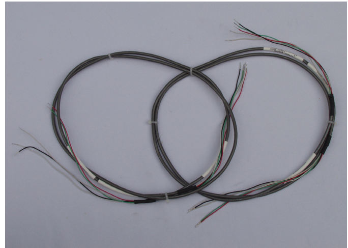
The MUXSIGNAL and MUXPOWER cables are typically used to attach the AM16/32B to the datalogger and power supply.
