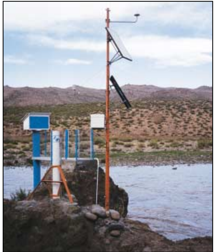
The INMARSAT-C satellite system provides telecommunications for remote Argentine stations where phone lines are impractical.
