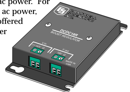
When using vehicle power, our DCDC18R Boost Regulator increases the vehicle's supply voltage to charging levels required by the CR5000.
