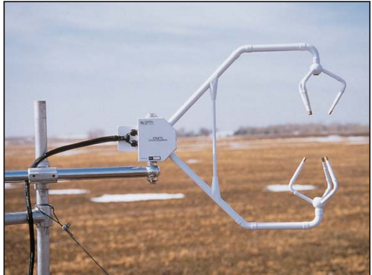
The CSAT3, shown making measurements over a fallow field in Minnesota, provides precision turbulence measurements with minimal flow distortion.
