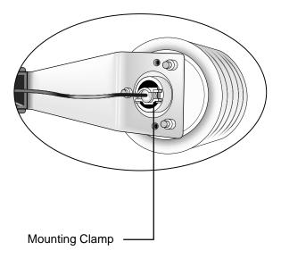
FIGURE 2. CS500 and 41301 Radiation Shield
