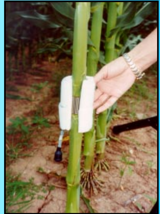
Each Dynagage sensor includes reference thermocouples, a thermopile, heating strip, foam insulation and a reflective weather shield to eliminate external thermal gradients.
