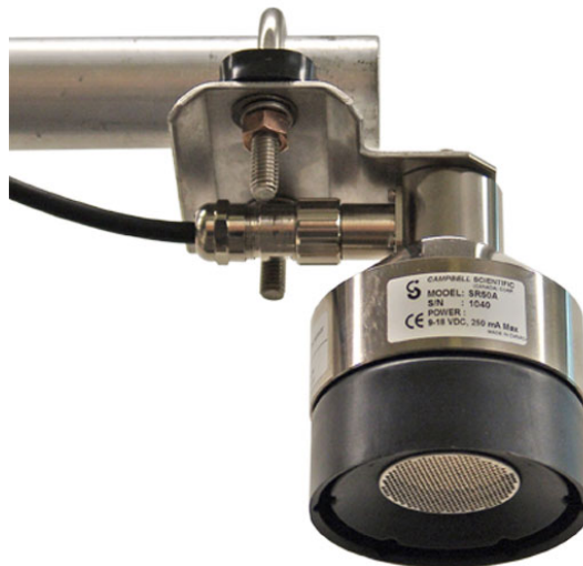
FIGURE 5. The SR50A Mounted to the Crossarm Shown from Another Angle
