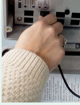
Expanding or reconfiguring the HOBO Weather Station or HOBO Micro Station is as simple as plugging in, or unplugging, smart sensors.
